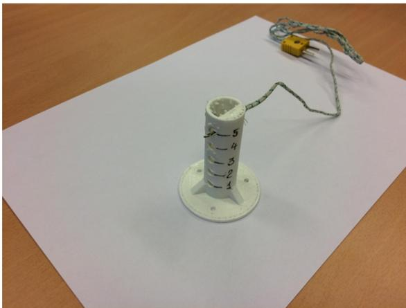
Figure 2. First testing version of the thermocouple
