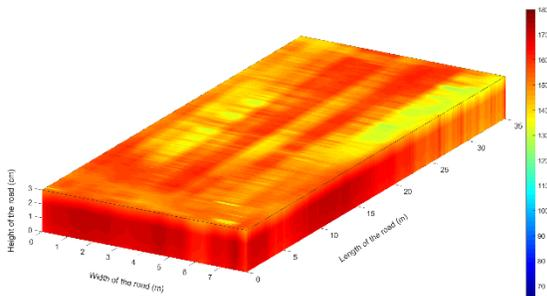
Figure 1. 3D asphalt temperature profile
